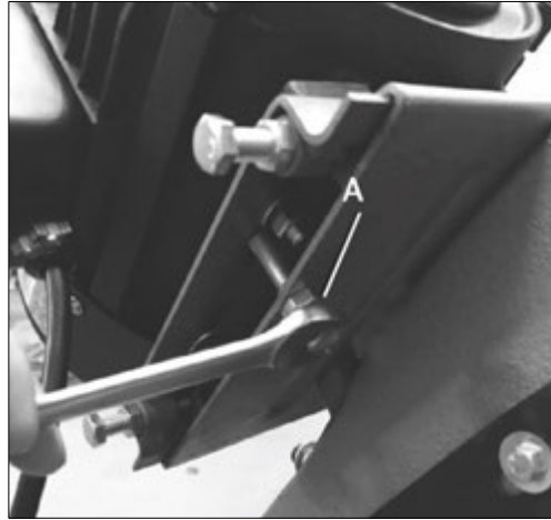
Figure 6-8: Tighten 5/16" Hex Screw
