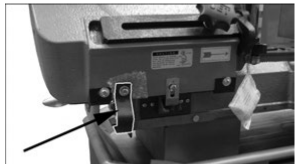
Figure 6-4: Shipping Bracket Removal
