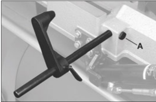
Figure 6-6: Installing Work Stop
