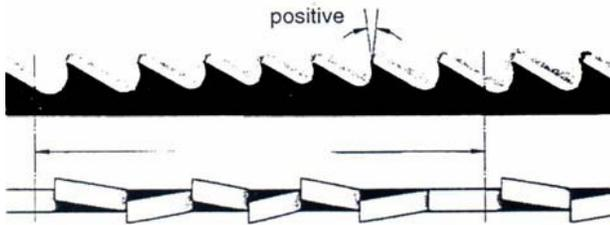
This type of blade is the most suitable for the cutting of section bars and large and thick pipes as well as for the cutting of solid bars at maximum machine capacity. Available pitches: 3-4/4-6.
