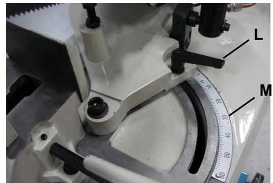
**⚠ CAUTION:** Check that the saw blade clears all parts of the vise assembly before cutting. The blade can strike parts of the assembly (especially during miter cuts) if not properly adjusted.
