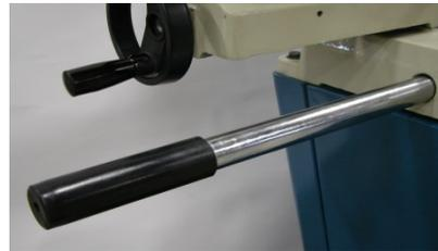
**⚠ CAUTION:** Make sure saw bow is in a down or horizontal position before moving or mitering to avoid tipping over machine.
