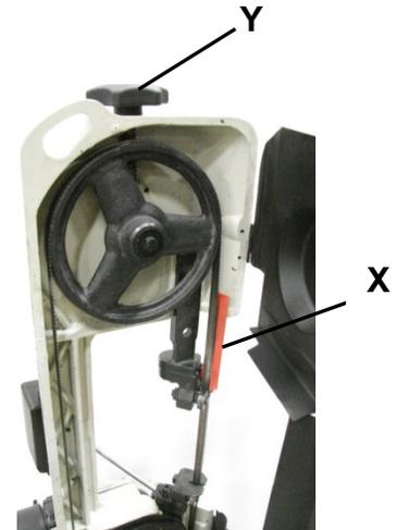
4. Install the new blade as follows with teeth slanting towards the motor.
