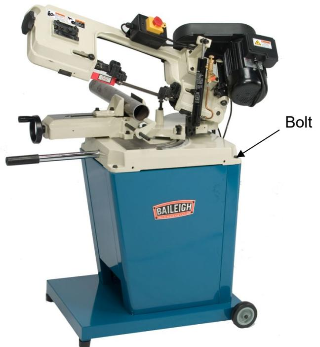
4. Attach the stop bar to the base as shown and tighten setscrew. (Can also be mounted on left hand side.)
