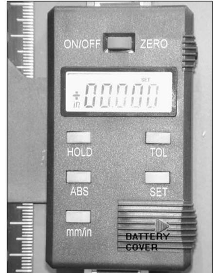
1. Press and hold the SET button until the '+' sign starts to flash and immediately release it.
