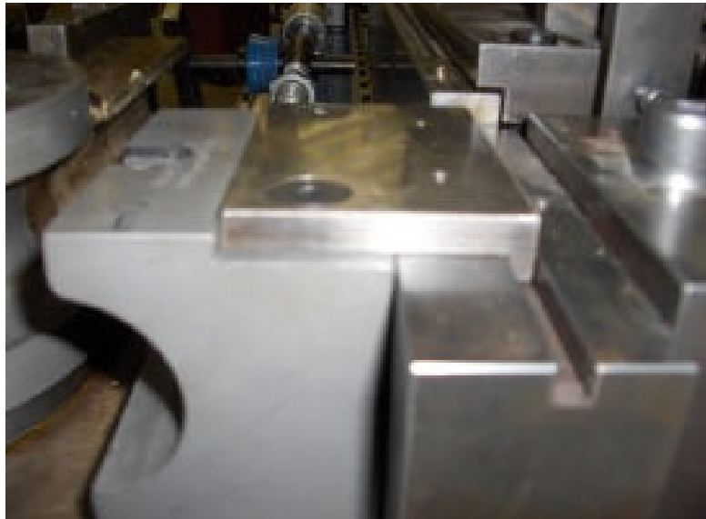
Figure 16 Clamp Die Holder is fully Seated
