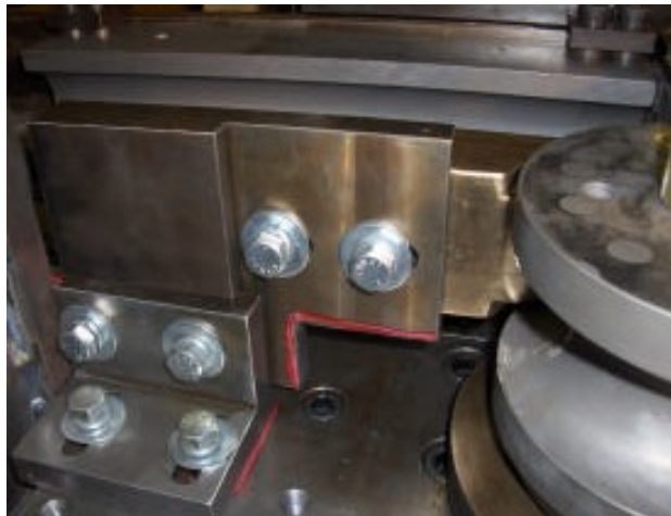
Figure 20 Installing Mounting Brackets
