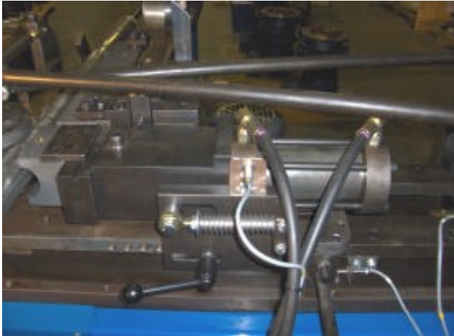
Figure 11 Clamp die Carriage in Home Position
