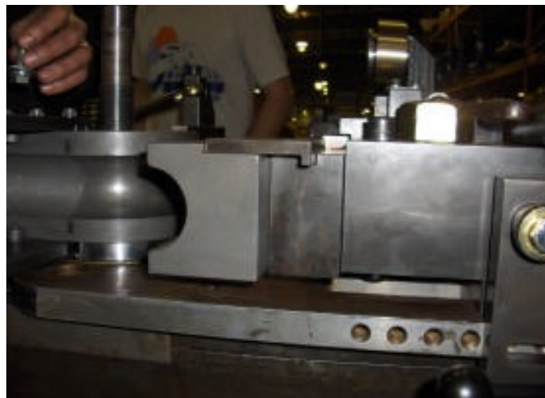
Figure 17 Clamp Die is not seated properly
