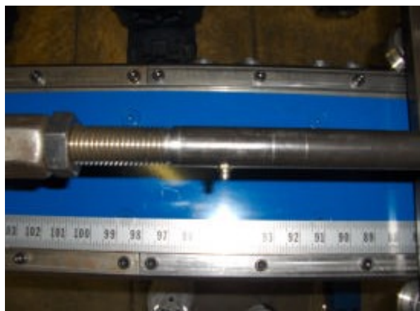
Figure 25 Greasing Mandrel via Zerk Fitting
