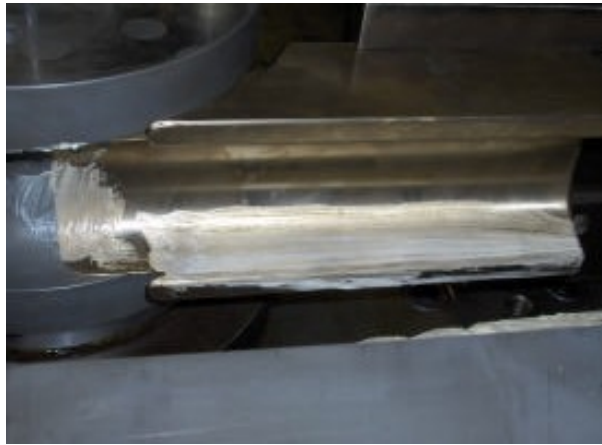
Figure 24 Applying Lubrication to the Wiper Die
