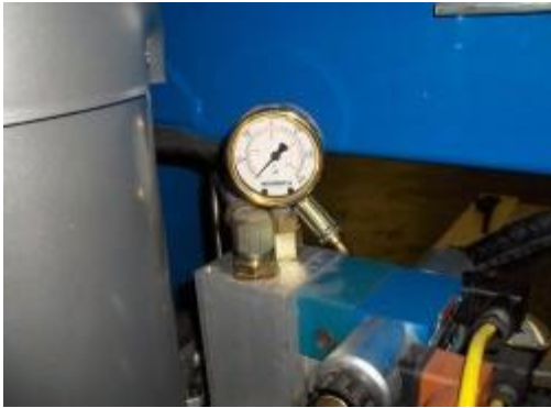
Figure 2 System pressure gauge Figure 3 Clamp Die Pressure Gauge
