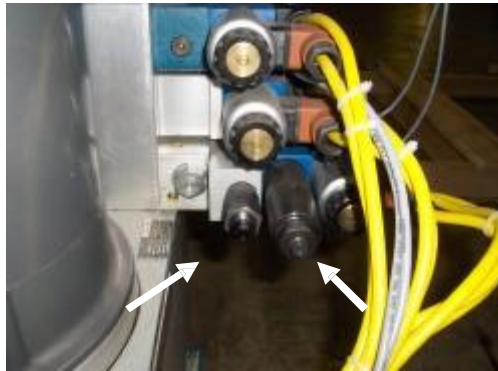
Figure 4 Pressure adjusting screws
