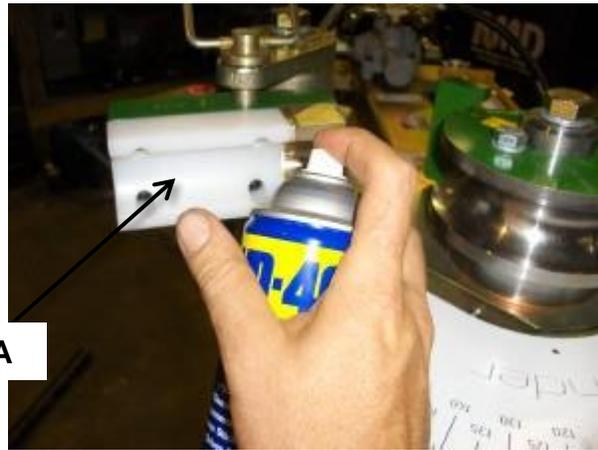
Lubricating counter die bending
